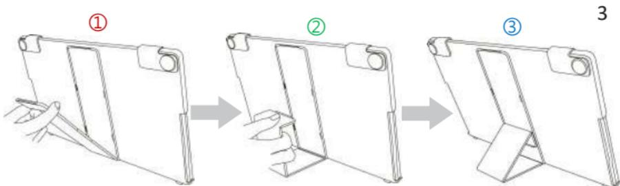
**⚠** The min. viewing angle of horizontal display is 40 degrees. Do not attach the rubber side of the magnetic buckle higher than 12cm from the bottom of the sheet mental, otherwise it may cause the monitor overturning.
