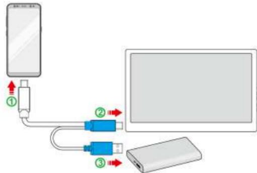
**Notice: You should deliver power current to On-Lap1306 in step 3. If the current is supplied to On-Lap 1306 by step 1 or 2, the monitor would be turned on before the smartphone is ready to transmit signals in time. This will result in video connection fail in DP Alt mode.**
