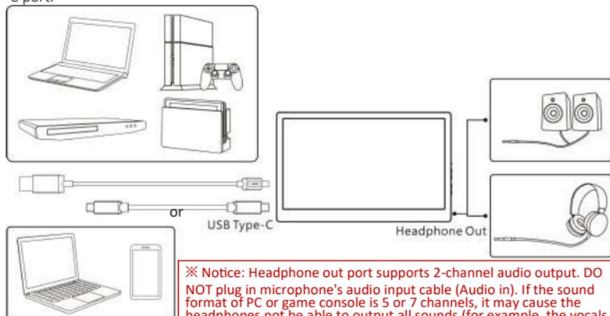
**※ Notice: Headphone out port supports 2-channel audio output. DO NOT plug in microphone's audio input cable (Audio in). If the sound format of PC or game console is 5 or 7 channels, it may cause the headphones not be able to output all sounds (for example, the vocals disappear in the game). Please select 2-channel audio output in sound settings of PC or game console.**
