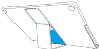
**⚠** The min. viewing angle of horizontal display is 40 degrees.
